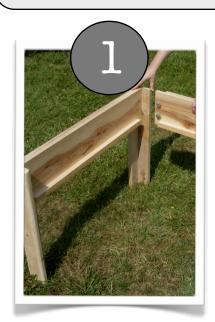
1) Connect (**B**) stringer leg to Leg end (**A**) using a 1/2 wrench with SMALL bolts until snug.
