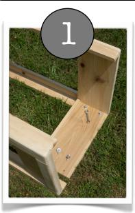
Lay (B) side legs on edge, span the bolt holes with (C) sides and tighten with 1/2 wrench until snug.
