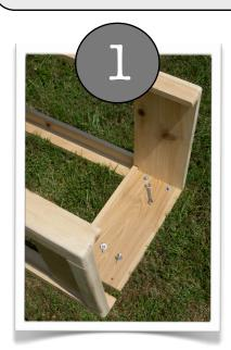
1) Lay (**B**) side legs on edge, span the bolt holes with (**C**) sides and tighten with 1/2 wrench until snug.
